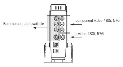
• A signal received at the **Flea** component input in 480p, 720p and 1080i, will only go out from the component output, in the same format.
